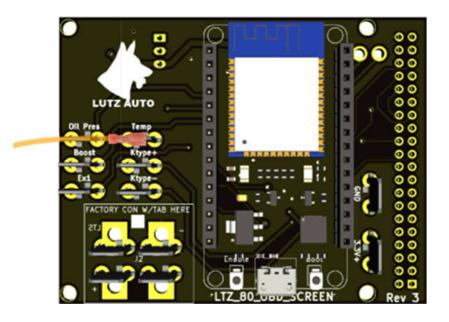
The supplied orange wire and spade connectors should be used to connect the "Temp" spade from the back of the multigauge to the temperature sensor.
