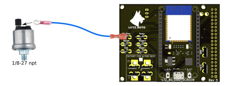
The red wire on the pigtail connector will need to be extended with the supplied red wire and run to the "3.3V+" Spade on the rear of the multigauge unit.
